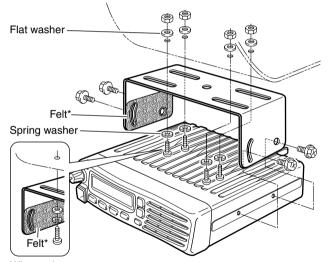
When using self-tapping screws
